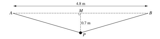
A particle P of mass 0.35 kg is attached to the mid-point of a light elastic string of natural length 4 m. The ends of the string are attached to fixed points A and B which are 4.8 m apart at the same horizontal level. P hangs in equilibrium at a point 0.7 m vertically below the mid-point M of AB (see diagram).
