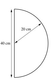
A frame consists of a uniform semicircular wire of radius 20 cm and mass 2 kg, and a uniform straight wire of length 40 cm and mass 0.9 kg. The ends of the semicircular wire are attached to the ends of the straight wire (see diagram). Find the distance of the centre of mass of the frame from the straight wire. [4]
